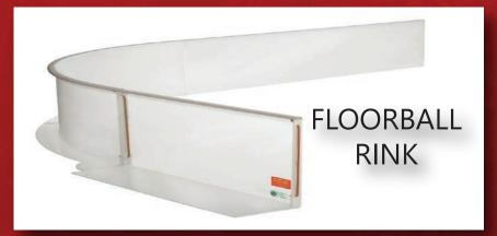
5 mm polypropylene bended in the bottom edge from one sheet without welding between the horizontal and vertical part All the pieces are long 2 or 1 meter and high 0,5 m. The top bar is made by a rounded resistent 15 mm polypropylene bar
